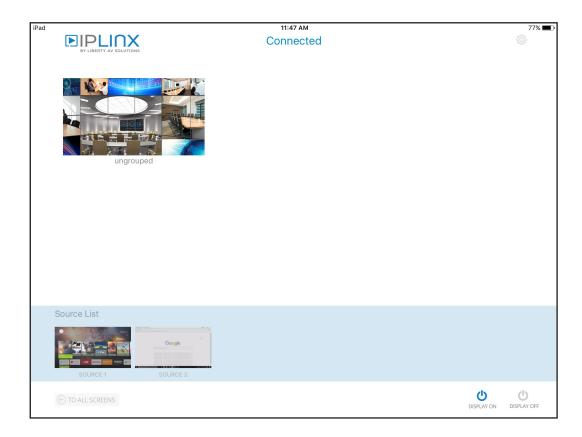
Groups (groups of displays, video wall configurations and their respective layouts) will be located in the upper half of the APP and sources will be located at the bottom half of the APP. Thumbnail previews of live sources in the A/V network will also appear in the respective source and displays lists in the APP.
